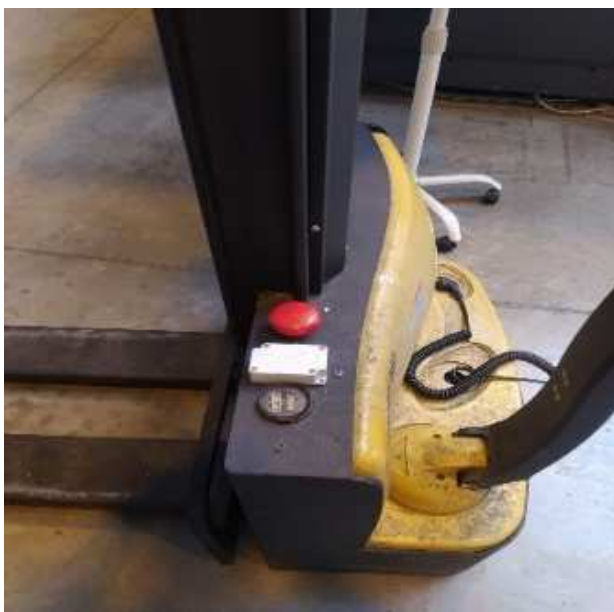
Figure 5 Installation of RTLS tag on the pallet truck
