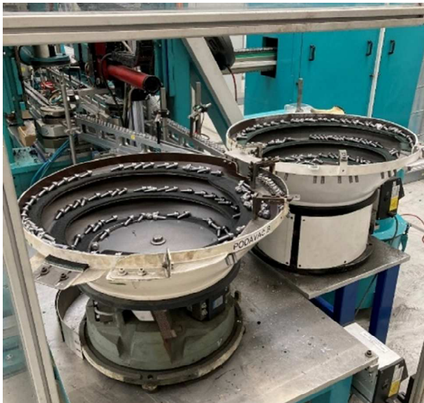
Figure 2 Vibratory bowl feeder
