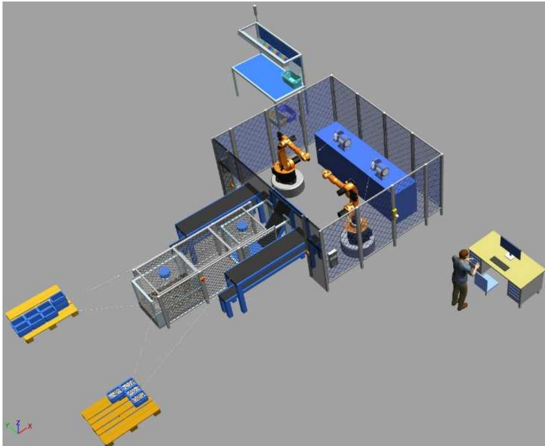
Figure 4 Simulation of the proposed polishing center
