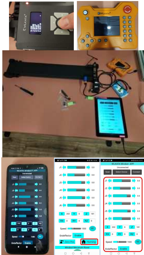
Figure 3 Accessories for controlling the Wlkata Mirobot (controller of the robot, universal controller for the robot or lunar vehicle via Bluetooth, control of movements via an application on a tablet and phone)
