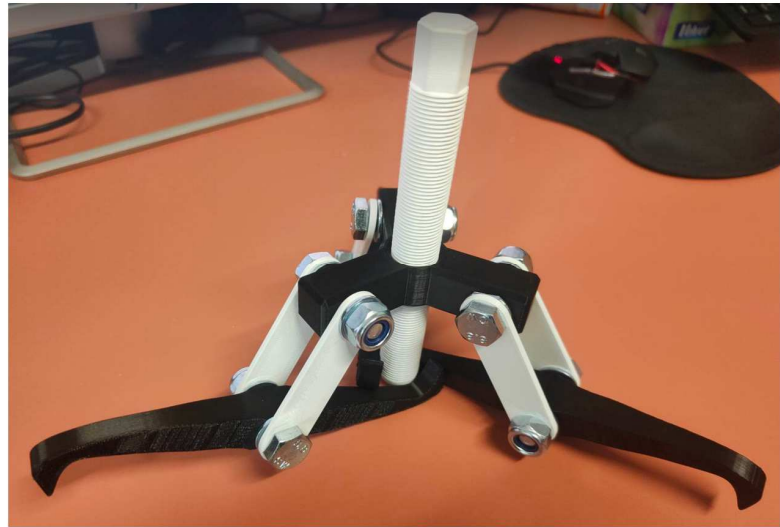
Figure 7 3D printing of a bearing puller
