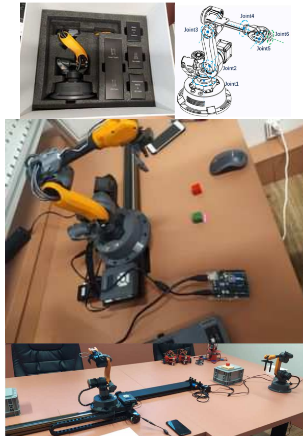
Figure 1 Wlkata Mirobot with 6 degrees of freedom designation
