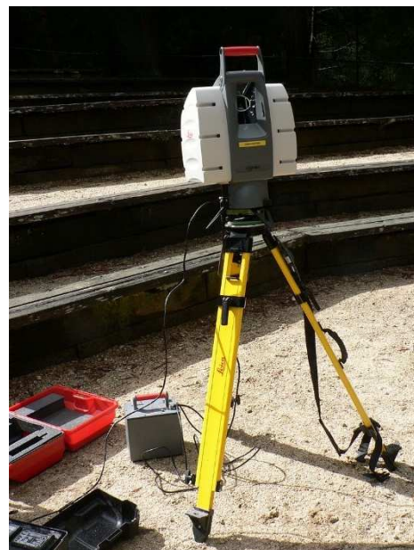
Figure 2 Lidar scanner for scanning buildings rock formations, etc. [2]
