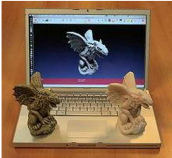
Figure 5 An example of real object replication by Means of 3D scanning and 3D printing
