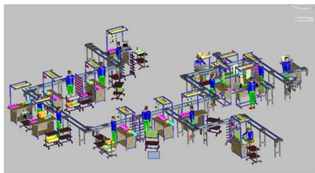
Figure 4 Examples of a draft concept for workplace work standing up and a seated position
